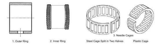
NIBL Bottom Roller Bearings – UN series are specially constructed Needle Roller Bearings for long and trouble free service. Every component of the bearing is manufactured to strict quality norms.
